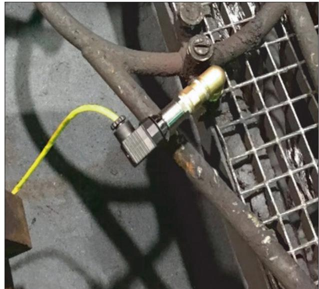
Fig. 3. Electronics pressure sensor connected to cooling ring of push bench [11]
