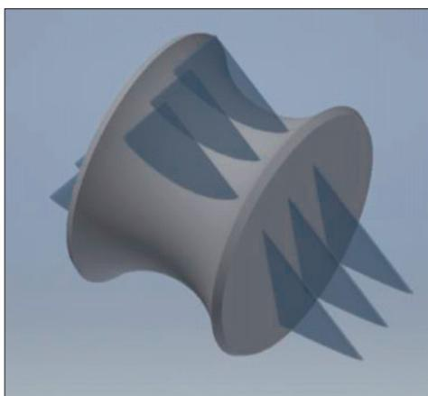
Fig. 4. Location of currently used flat nozzles [13]
