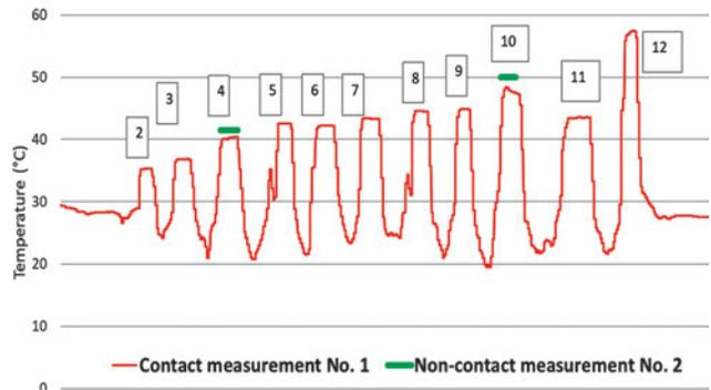
**Fig. 6. Rolls surface temperature of the rolls in the push bench**
